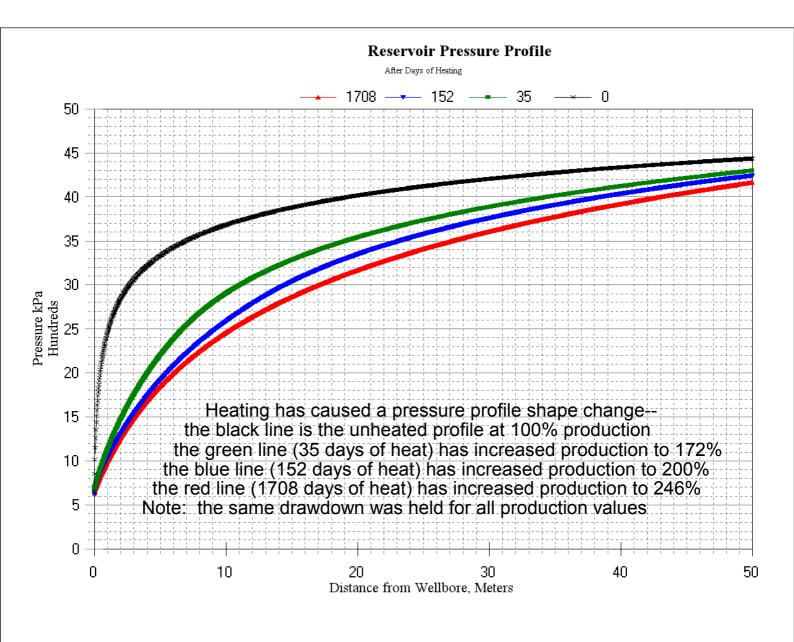
**PEPS** plots the pressure for each hollow cylindrical shell, calculates how many days of heating are needed to reach the increased production, and generate a "Reservoir Pressure Profile"
