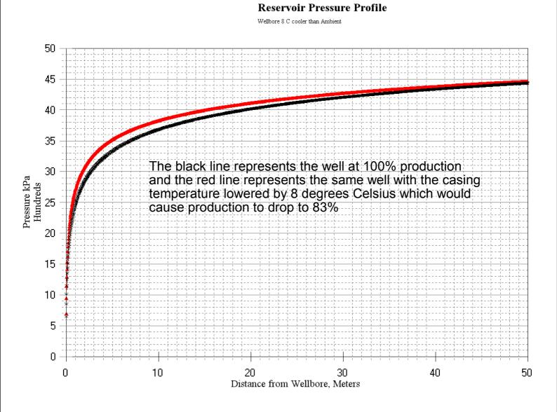
The exact nature of the lower temperature is not fully confirmed but gas expansion is suspected as a "lower than normal" bottom hole temperature has not been observed on wells without noticeable gas. A good example of production cooling and the increase due to heating is given by the PEPS projection below and SPE paper SPE68220 on Bahrain well 480.
