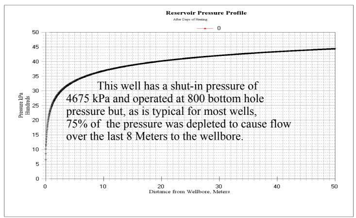
Any flow enhancement made in the near wellbore will cause a substantial improvement in production
