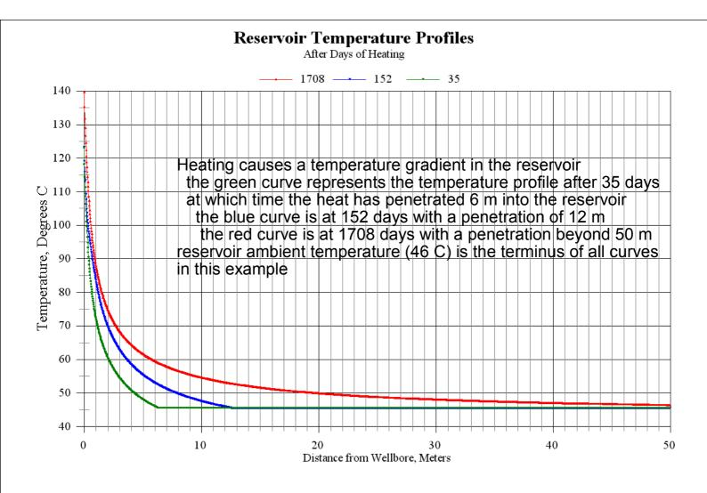
To generate the profiles the program inputs (heating power and increased production) are increased to bring the casing temperature up to 120 to 130 Celsius with the same drawdown as existed in the unheated well
